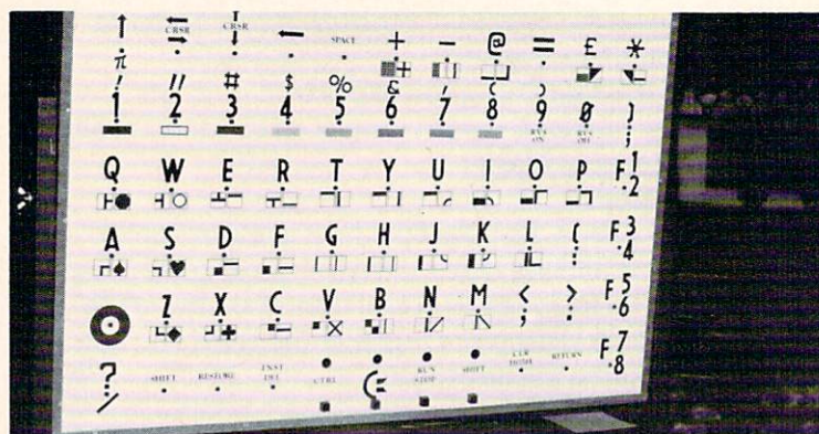
Jerry Oberwager's computerized letterboard began as a simple “spelling machine”. Below each “key” on the board is a tiny photoelectric cell.
